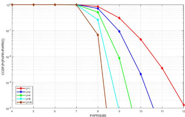
Fig. 8. PAPR of OFDM signal with SLM,  $N=512$ ,  $U=1,2,4,8,16$ .
