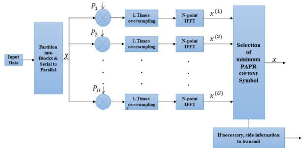
Fig. 2. The framework of selective mapping.
