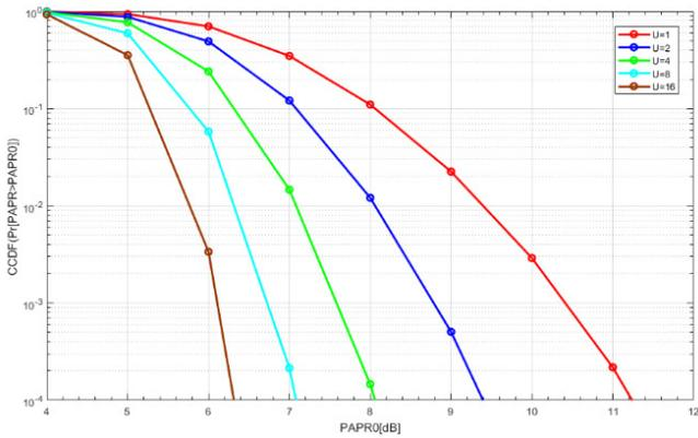
Fig. 6. PAPR of OFDM signal with SLM,  $N=128$ ,  $U=1,2,4,8,16$ .
