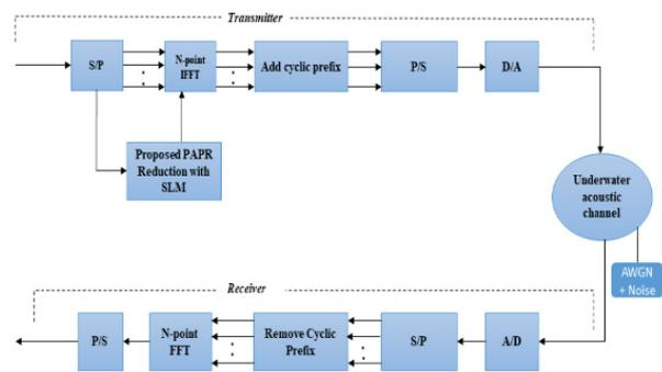
Fig. 1. The framework of UWA OFDM communication system.
