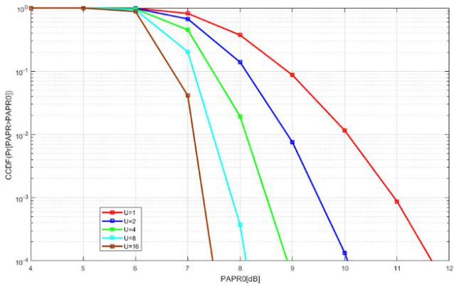
Fig. 7. PAPR of OFDM signal with SLM,  $N=256$ ,  $U=1,2,4,8,16$ .
