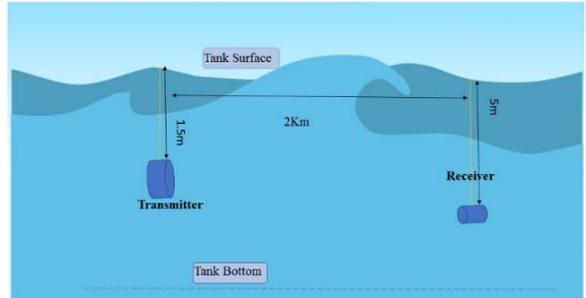
Fig. 3. Schematic layout of UWA communication with single transducer and a single hydrophone.
