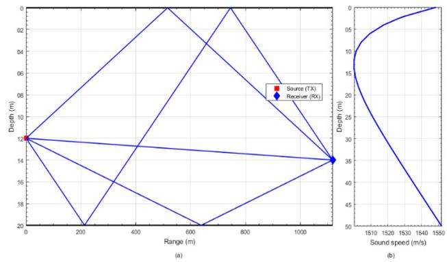
Fig. 4. (a) Multipath channel Eigen ray, (b) sound speed profile in the water.
