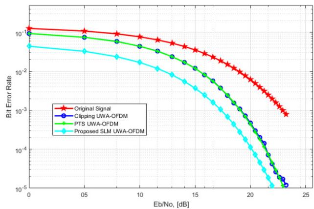
Fig. 9. BER vs signal to noise ratio for QPSK modulation in the Bellhop channel.
