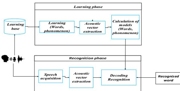
Fig. 3. The modified speech recognition system.
