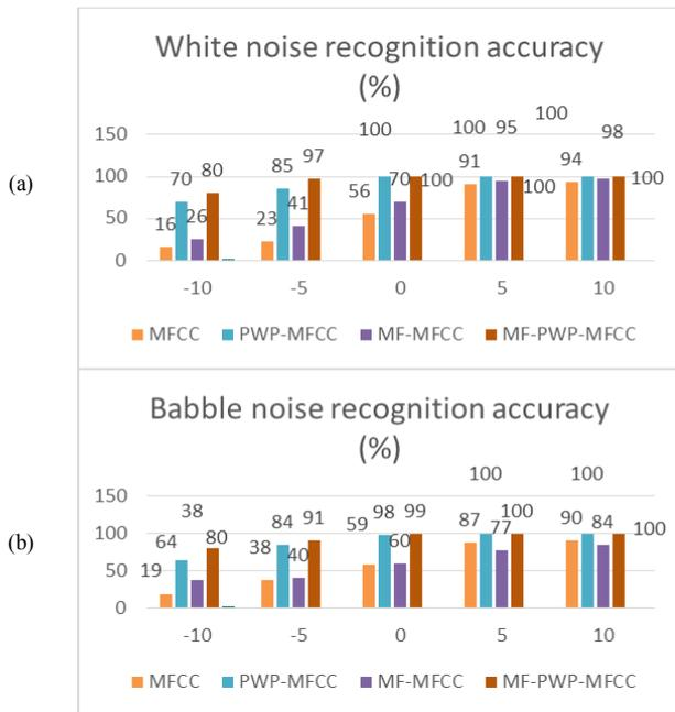
Fig. 4. Comparison of recognition accuracy in: (a) white noise and (b) babble noise for several feature extraction methods.
