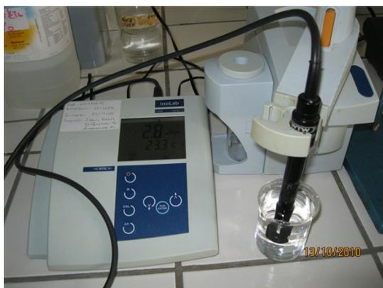
Fig. 4. Device for conductivity measurements
