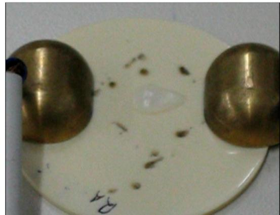
Fig. 9. Droplet deformation under the influence of electric field
