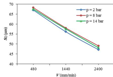
Fig. 3.  $S_z$  as a function of  $V$  for three values of  $p$ .
