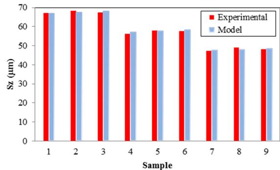
Fig. 7. Comparison between experimental and predicted data for maximum surface roughness.
