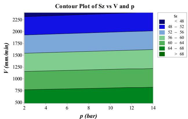
Fig. 9. Contour plot of surface roughness  $S_z$  versus cutting speed  $V$  and assist-gas pressure  $p$ .
