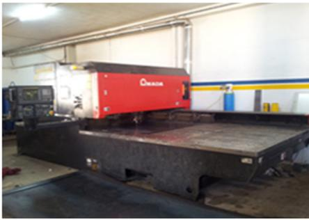
Fig. 1. The laser cutting machine AMADA AS 4000 E.
