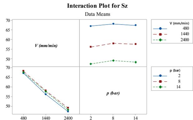
Fig. 8. Interaction plot showing the effects of cutting speed  $V$  and assist-gas pressure  $p$  on surface roughness  $S_z$ .
