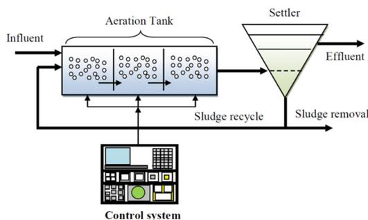
Fig. 5. Schema of activated sludge process.
