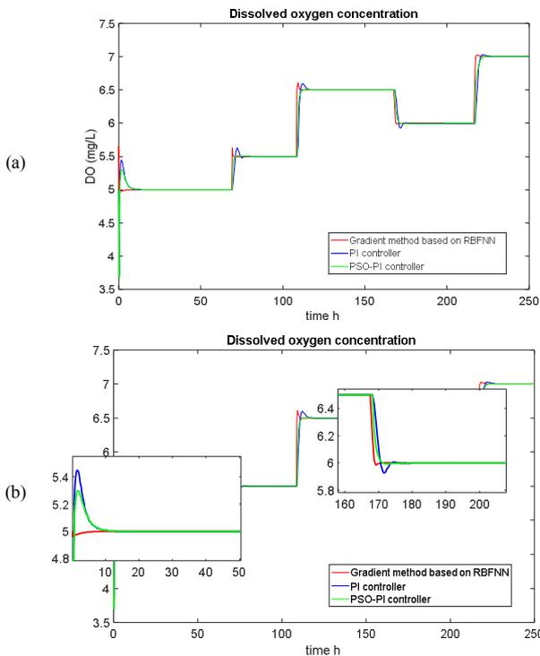
Fig. 8. a) Dissolved oxygen concentration with constant dilution rate  $D=0.04h^{-1}$ , b) zoomed view.
