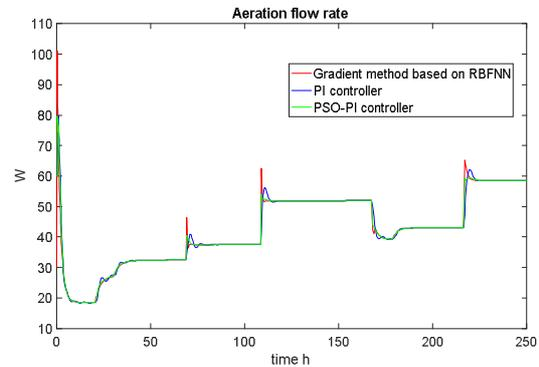
Fig. 13. Aeration rate (control variable).
