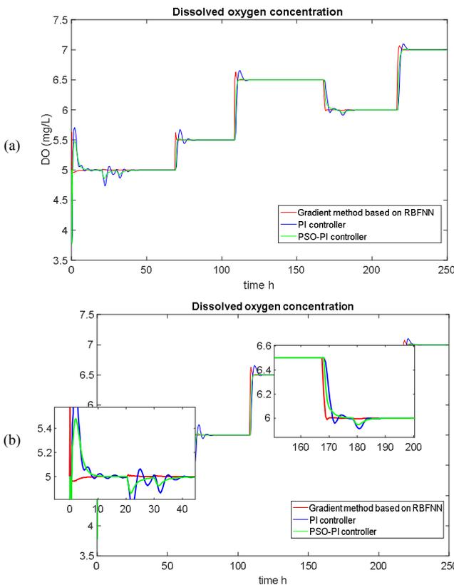
Fig. 12. a) Dissolved oxygen concentration with modified dilution rate and influent substrate, b) zoomed view.
