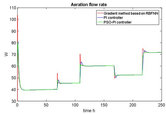
Fig. 9. Aeration rate (control variable).
