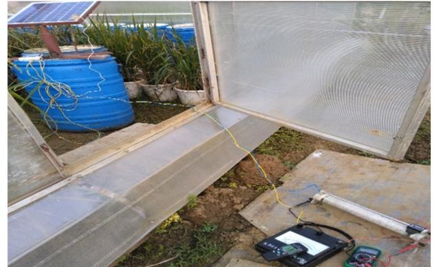
Fig. 4. Solar PV Panel under OTC 1 with 575ppm CO<sub>2</sub> concentration.
