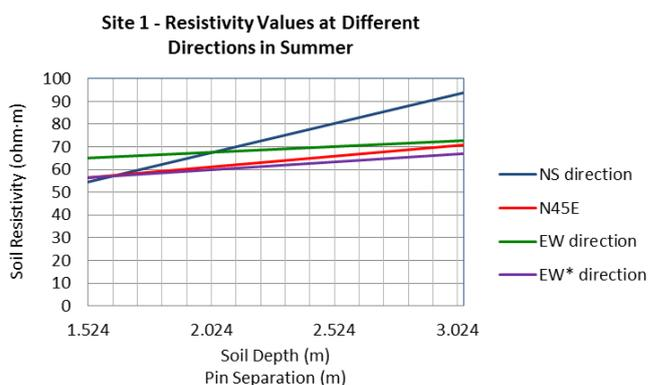
Fig. 4. Resistivity values in site 1 measured in different directions in summer. The EW\* direction means that measurements were taken where the profile runs along a dug and refilled utility trench of 4 feet deep.
