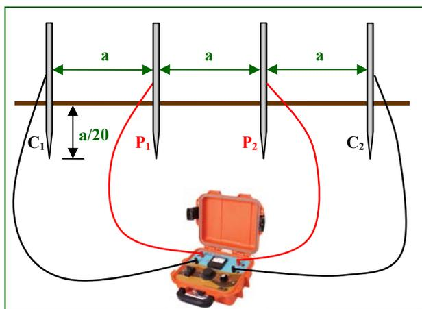
Fig. 1. Wenner array. The resistivity meter used is Model H-4385 made by Humboldt MFG©
