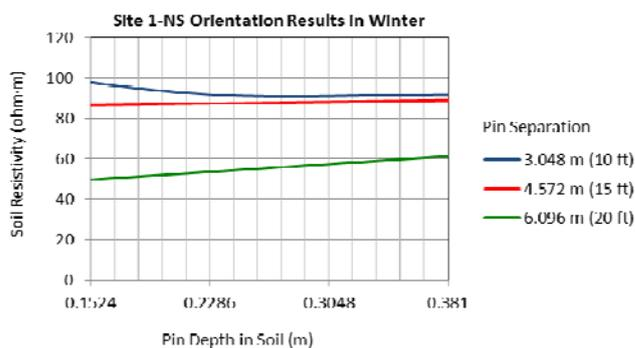
Fig. 2. Resistivity values in site 1 measured in the NS direction in winter.
