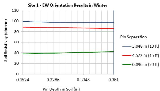
Fig. 3. Resistivity values in site 1 measured in the EW direction in winter.
