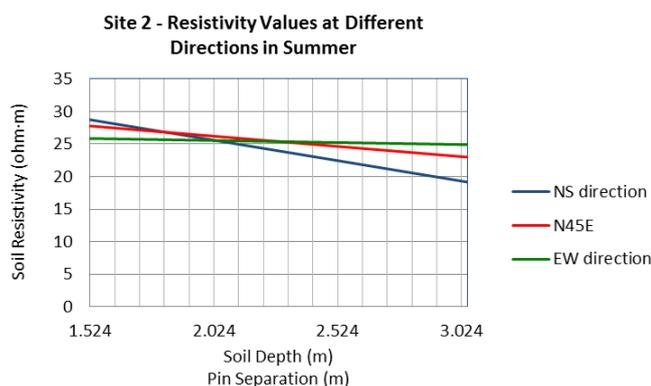
Fig. 5. Resistivity values in site 2 measured in different directions in summer.
