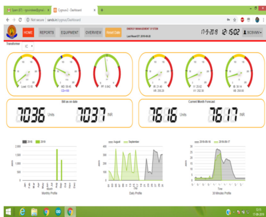
Fig. 8. Real time energy monitoring live report from the cloud
