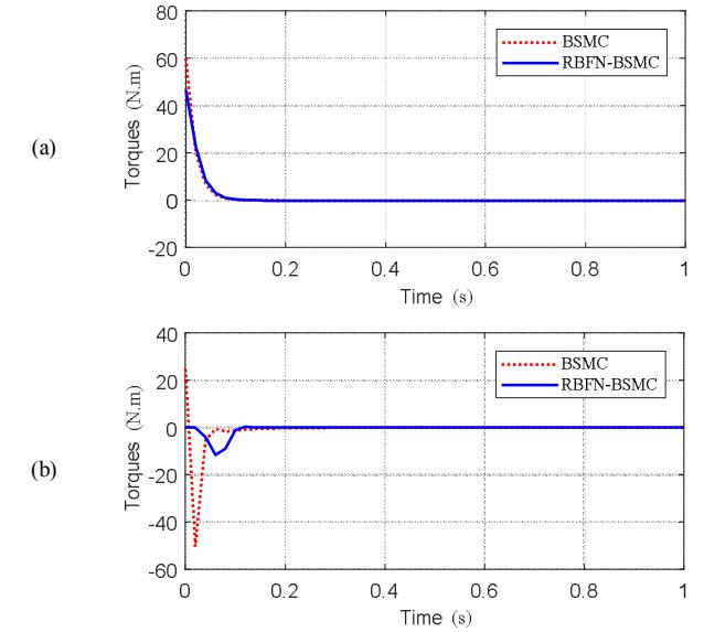
Fig. 4. Input torques with constant roll inertial. (a) Rewinding roll, (b) unwinding roll
