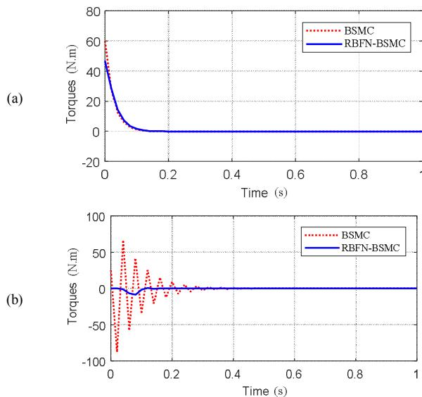
Fig. 7. Input torques with varying roll inertia. (a) Rewinding roll, (b) unwinding roll
