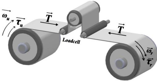
Fig. 1. Single-span web control system
