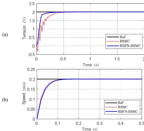
Fig. 6. System response with varying roll inertia. (a) Web tension, (b) web speed
