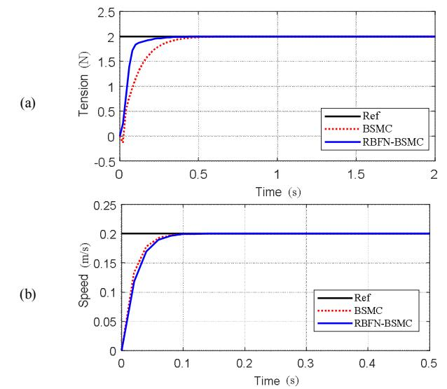
Fig. 3. System response with constant roll inertia. (a) Web tension, (b) web speed
