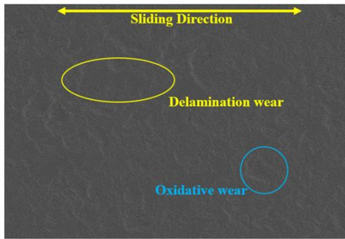
Fig. 11. SEM image of heat-treated specimens at  $\times 500$  for B2 (layer thickness: B2=10.4 $\mu\text{m}$ )
