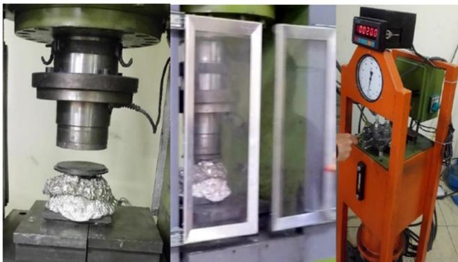
Fig. 1. Pressing and heating of the Ti-6-4 powder
