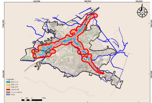
Fig. 24. Flood area mapping of Oued Batna and Oued El Gourzi valleys based on 100-year frequency flow – under ArcGIS 10.3
