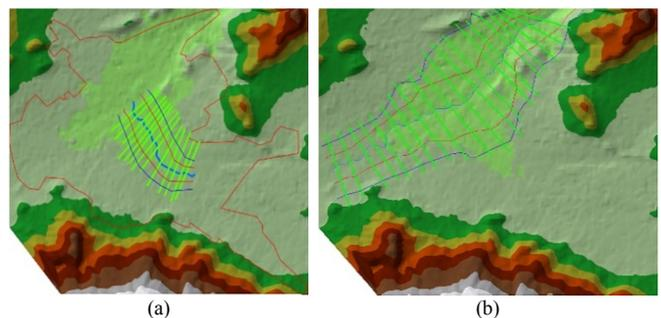
Fig. 18. Extraction of geometric data using HEC GeoRAS of the valleys Oued Batna and Oued El Gourzi
