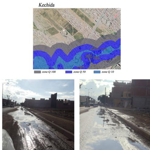
Fig. 26. Areas exposed to flooding risk at the level of Kechida Road
