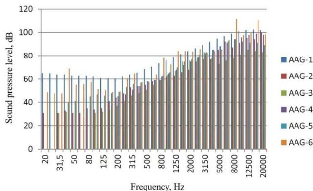
Fig. 9. The sound pressure levels of acoustic field generated by acoustic generators
