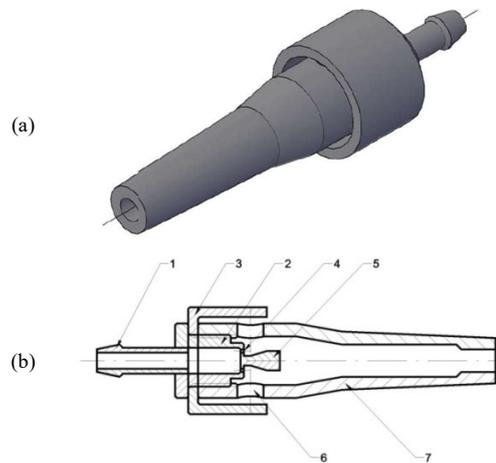
Fig. 3. Acoustic generator AAG-3: a) 3D model, b) longitudinal section
