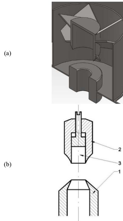
Fig. 6. Acoustic generator AAG-6: a) 3D model, b) longitudinal section
