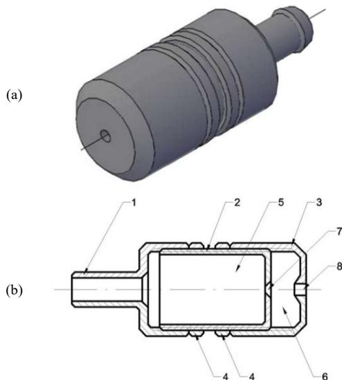
Fig. 2. Acoustic generator AAG-2: a) 3D model, b) longitudinal section
