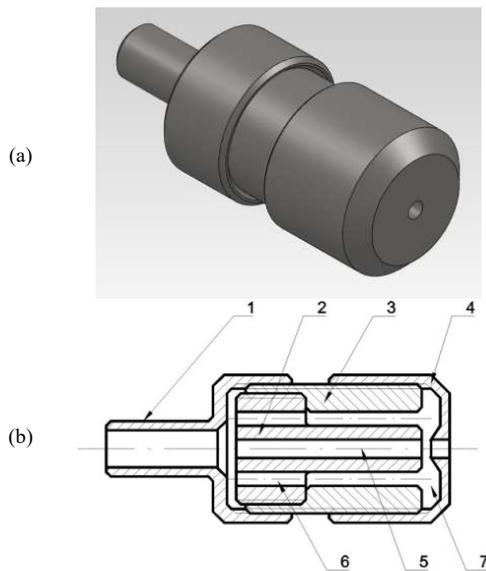
Fig. 1. Acoustic generator AAG-1: a) 3D model, b) longitudinal section
