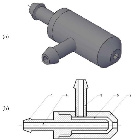
Fig. 4. Acoustic generator AAG-4: a) 3D model, b) longitudinal section
