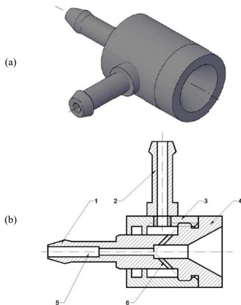
Fig. 5. Acoustic generator AAG-5: a) 3D model, b) longitudinal section
