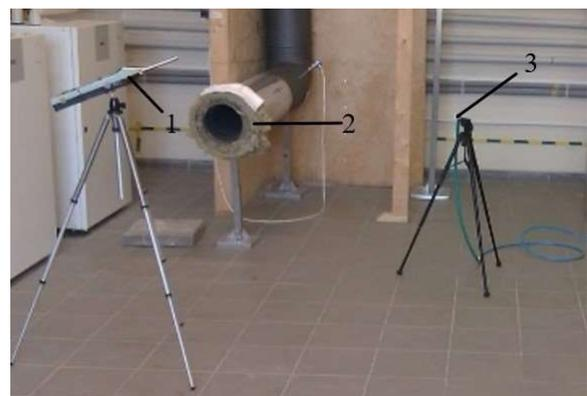
Fig. 7. Experimental setup. 1: sound level meter/analyzer, 2: acoustic chamber, 3: compressed air port
