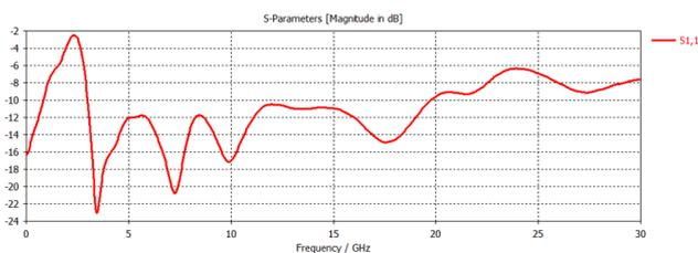
Fig. 2. Simulated reflection coefficient (S11) vs operating frequency
