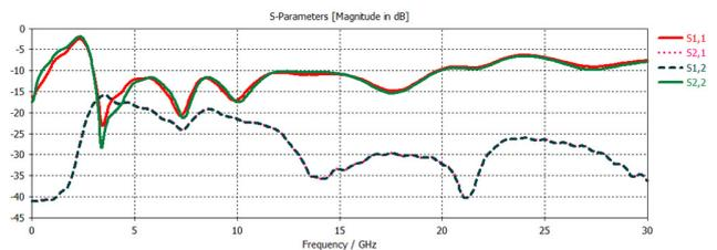
Fig. 6. Reflection and transmission coefficients for the monopole system vs operating frequency
