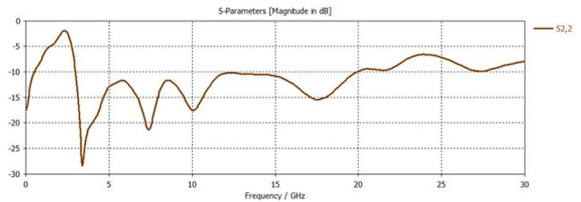
Fig. 3. Simulated reflection coefficient (S22) vs operating frequency
