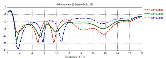
Fig. 4. Reflection coefficients for several values of feeding line width
