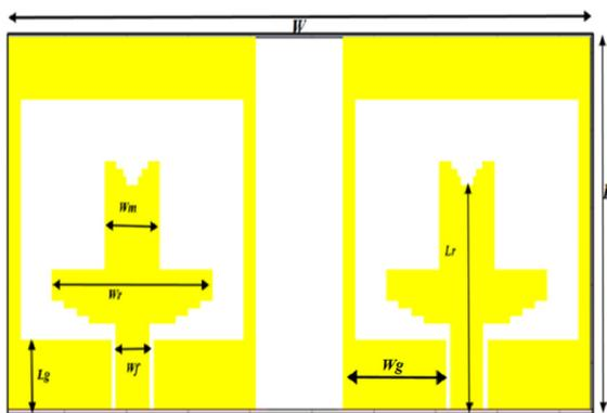
Fig. 1. Geometry of the proposed MIMO antenna
