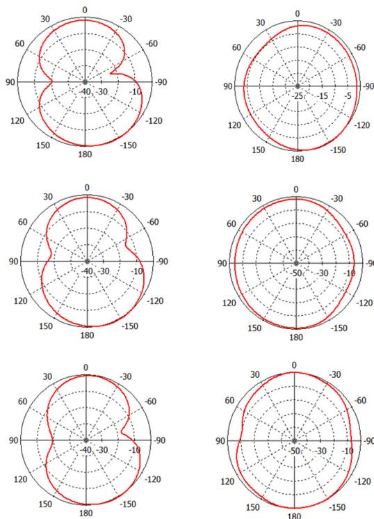
Fig. 7. Simulated power radiation pattern in polar form (elevation and azimuth planes) of the proposed MIMO antenna at 3.48GHz, 7.32GHz, 9.89GHz, and 17.62GHz
