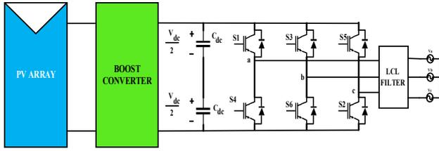
Fig. 1. Two-stage three-phase grid-connected PV system.
