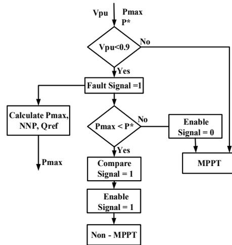
Fig. 2. Flowchart of the proposed control algorithm
