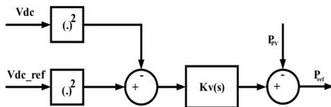
Fig. 3. Diagram control  $V_{dc}$  voltage
