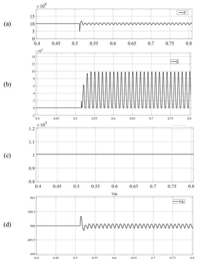
Fig. 8. The power output parameters of the system: a) active power injected to the grid, b) reactive power injected to the grid, c) active power reference, d) voltage of DC-link
