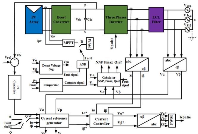
Fig. 4. Control structure of VSI [9] (the non MPPT mode is ignored)
