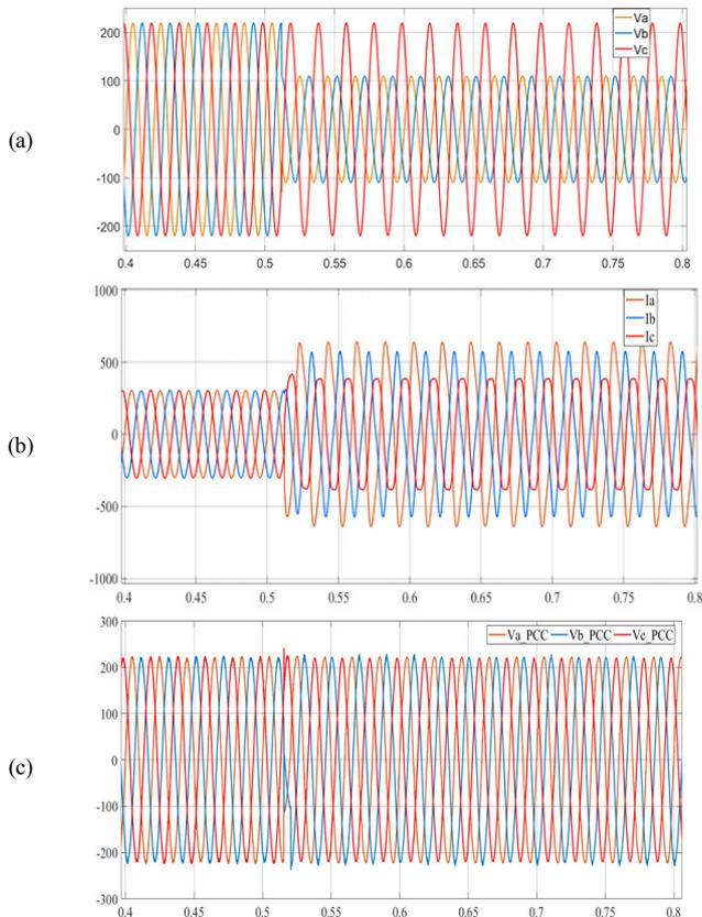
Fig. 7. Grid parameters: a) PCC voltage before injecting reference current, b) PV system current injected to the grid under fault occurrence, c) PCC voltage after injecting reference current
