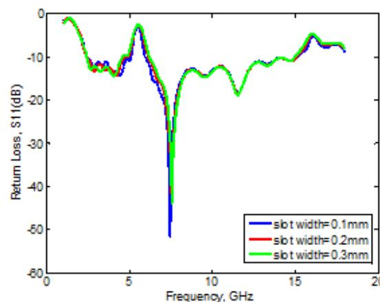
Fig. 5. Return losses of proposed antenna with slot width dimension of 0.1, 0.2, and 0.3mm respectively
