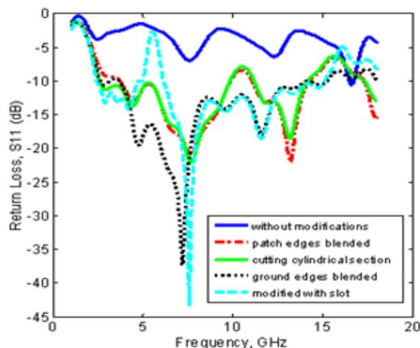
Fig. 2. Return losses for all modifications of the proposed antenna
