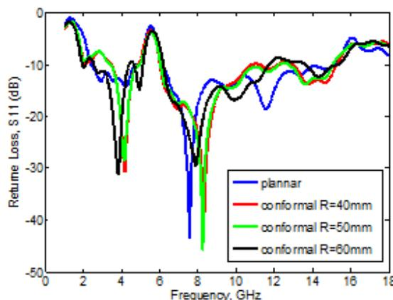
Fig. 4. Return losses of proposed antenna conformed on cylindrical substrates of radiuses; 40, 50 and 60 mm.
