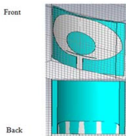
Fig. 3. 3D view of the proposed antenna conforming on cylindrical substrate, with front and back views
