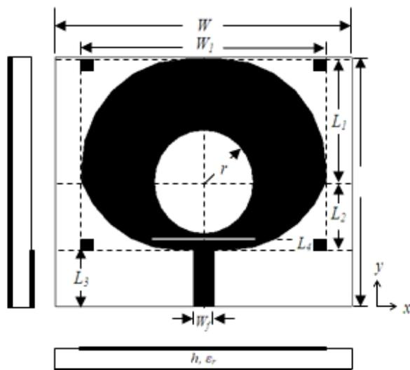
Fig. 1. The geometry of the proposed planar antenna
