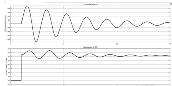
Fig. 10. Without PSS when 300MW load is connected
