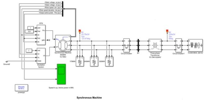
Fig. 2. MATLAB/Simulink model without PSS
