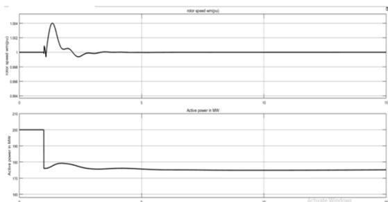
Fig. 13. Without PSS when 175MW load is connected
