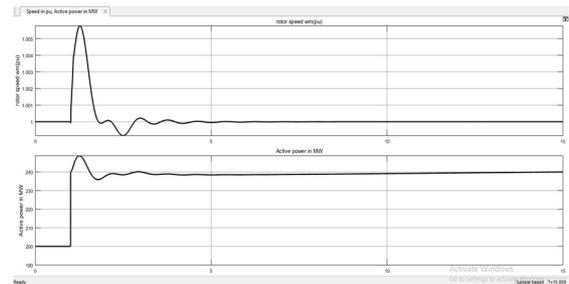
Fig. 9. With PSS when 240MW load is connected
