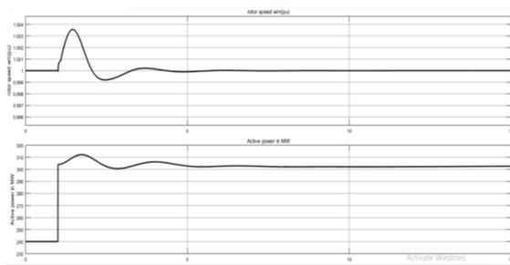
Fig. 11. With PSS when 300MW load is connected
