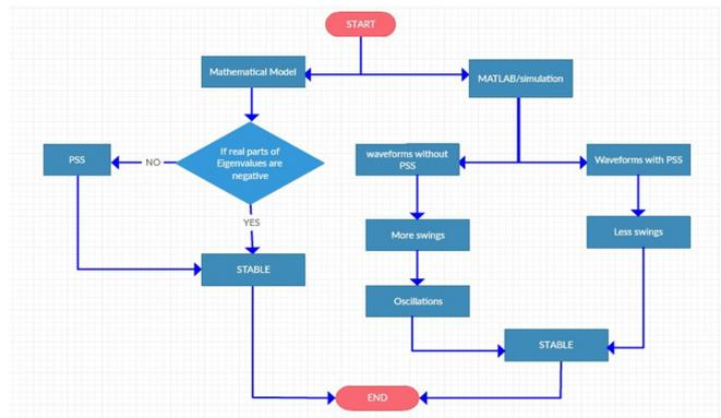
Fig. 1. Flow chart of the proposed identification by eigenvalues and PSS
