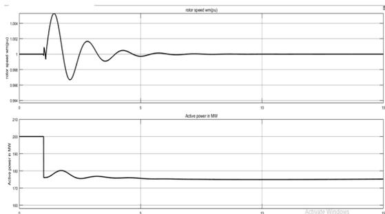
Fig. 12. Without PSS when 175MW load is connected
