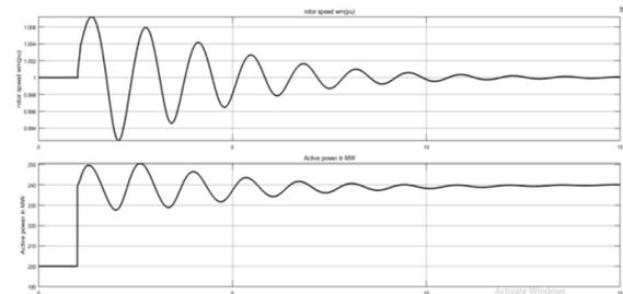
Fig. 8. Without PSS when 240MW load is connected
