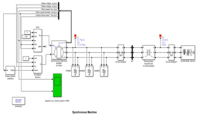
Fig. 3. MATLAB/Simulink model with PSS
