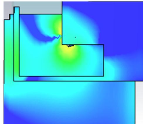
Fig. 12. Current distributions at the resonant frequency of 1800MHz
