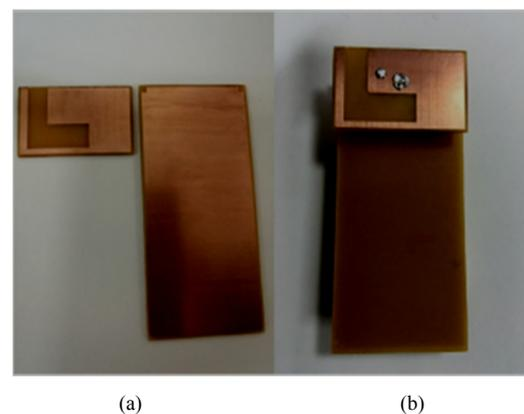
Fig. 9. Photos of the realized PIFA antenna: (a) before and (b) after assembly
