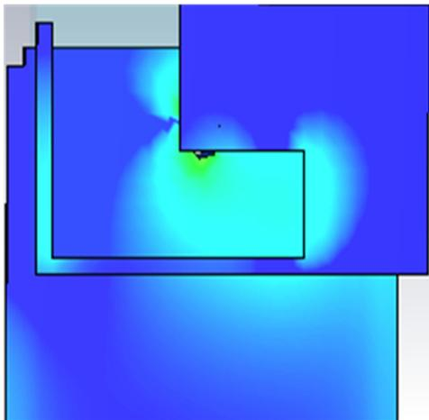
Fig. 11. Current distributions at resonant frequency 900MHz
