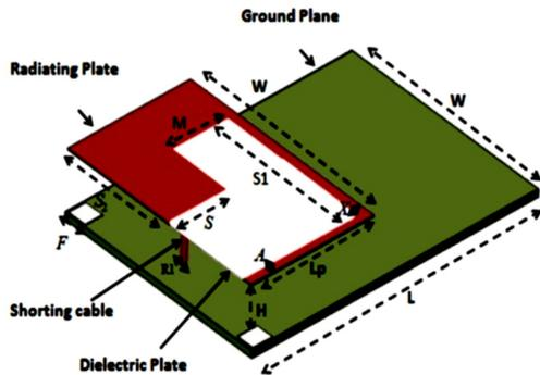
Fig. 1. Geometry of the proposed PIFA antenna
