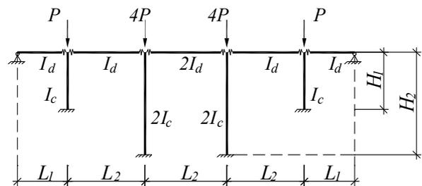
Fig. 3. Semi-rigid connection plane frame analysis
