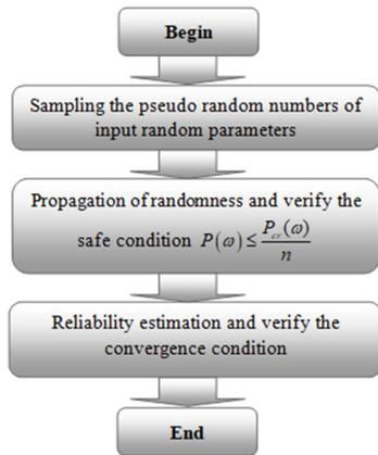
Fig. 1. Scheme of the reliability assessment of the steel frame considering semi-rigid connection using Monte Carlo simulation method
