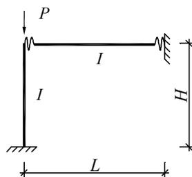
Fig. 2. Plane frame semi-rigid connections for validation
