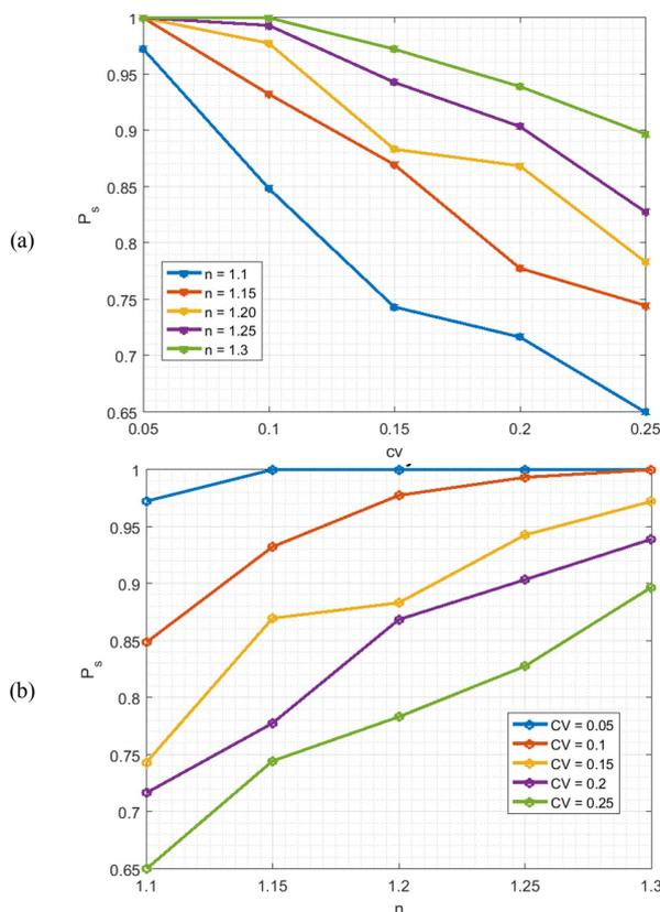
Fig. 5. (a) Effect of the coefficient of variation and (b) effect of the safety factor on the safe probability of the column
