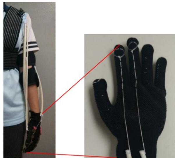
Fig. 1. Prototype exoskeleton with attached Dyneema fibre ongloves
