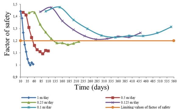
Fig. 13. Safety factor vs time at different rates of lowering of the reservoir, when the undrained shear strength of clay is  $30\text{kN/m}^2$
