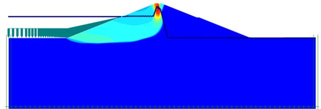
Fig. 14. Failure zone of the dam when the reservoir was lowered at a rate of 1m/day for a depth of 20m ( $S_u=30$ )
