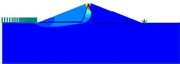
Fig. 12. Failure zone of the dam when the reservoir was lowered at a rate of 0.1m/day for a depth of 55m ( $S_u=25$ )
