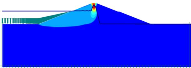
Fig. 11. Failure zone of the dam when the reservoir was lowered at a rate of 1m/day for a depth of 20m ( $S_u=25$ )
