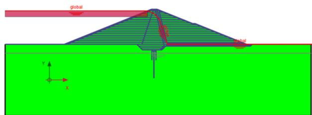
Fig. 3. 10m lowering of the reservoir at the rate of 1m/day
