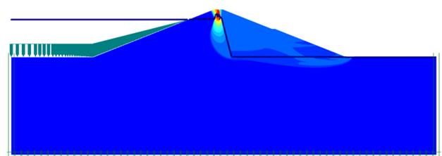
Fig. 8. Failure zone of the dam when the reservoir was lowered at a rate of 1m/day for a depth of 10m (Su=20)
