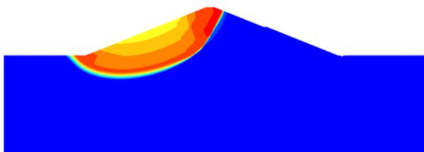
Fig. 5. Failure zone of the dam after the end of construction
