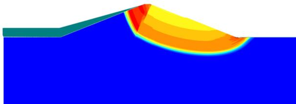
Fig. 6. Failure zone of the dam after the filling of the reservoir
