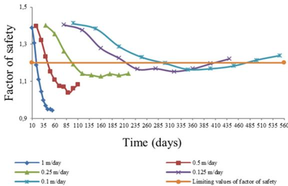
Fig. 10. Safety factor vs time at different rates of lowering of the reservoir, when the undrained shear strength of clay is  $25\text{kN/m}^2$
