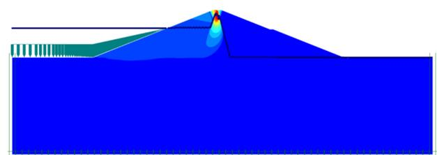
Fig. 9. Failure zone of the dam when the reservoir was lowered at a rate of 0.1m/day for a depth of 20m (Su=20)
