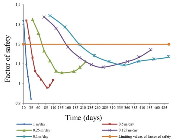
Fig. 7. Safety factor vs time at different rates of lowering of the reservoir, when the undrained shear strength of clay is 20kN/m<sup>2</sup>
