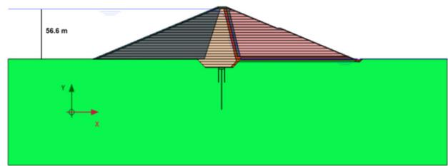
Fig. 2. High reservoir level location of the embankment dam
