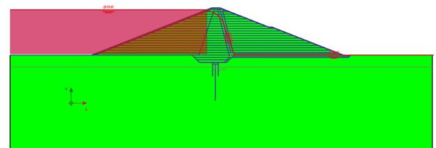
Fig. 4. A view of lowering of reservoir up to a depth of 55 m at 0.1 m/day
