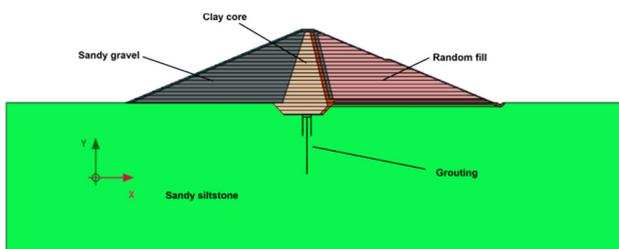
Fig. 1. Cross section of a rainfed embankment dam
