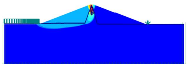
Fig. 15. Failure zone of the dam when the reservoir was lowered at a rate of 0.1m/day for a depth of 55m ( $S_u=30$ )
