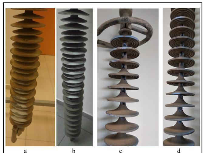
Fig. 1. Visible traces of flashover (discolored sheds) in a-b and flashunder (damaged sheath) in c-d. Photos a and b from past faults. Photos c and d from the insulator of the incident analyzed in this paper.
