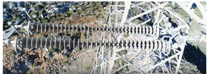
Fig. 4. The flashed under insulator with visible arc traces on rings. Sheath damage barely visible from this angle and distance.
