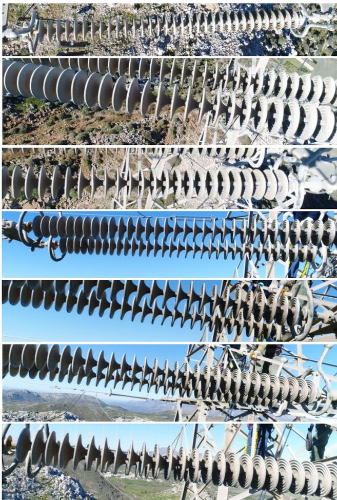
Fig. 10. Views of the flashed under insulator before its removal
