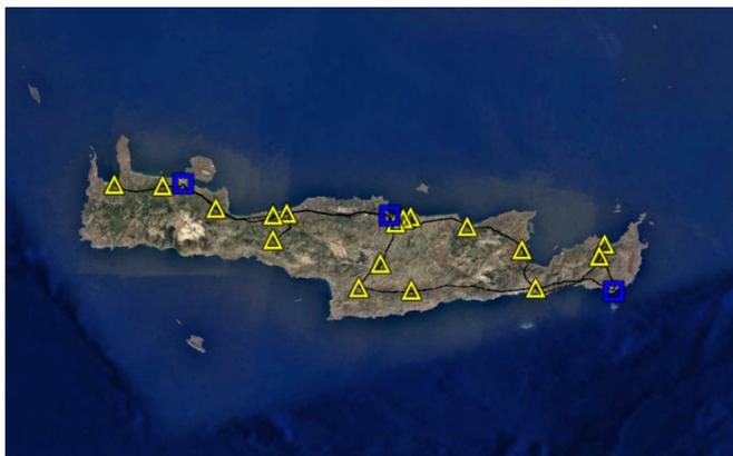
Fig. 2. The Transmission System of Crete (screenshot from Google Earth. Map data: Image LandSat/Copernicus) (yellow triangles: step-down substations, blue squares: step-up substations attached to power plants).
