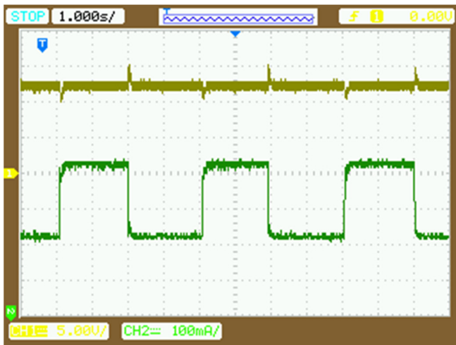
Fig. 6. Inductor current response (green line) and output voltage response (dark yellow line)
