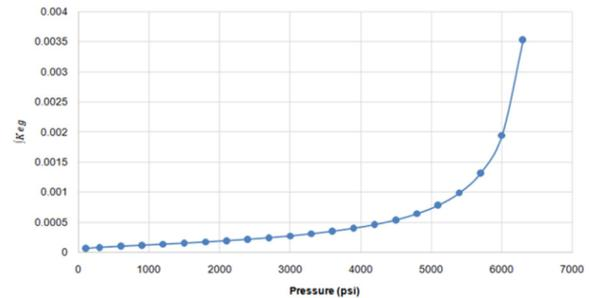
Fig. 4. Integral of effective permeability versus pressure at assumed pressure points
