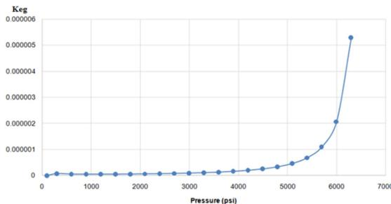
Fig. 6. Gas effective permeability vs. pressure
