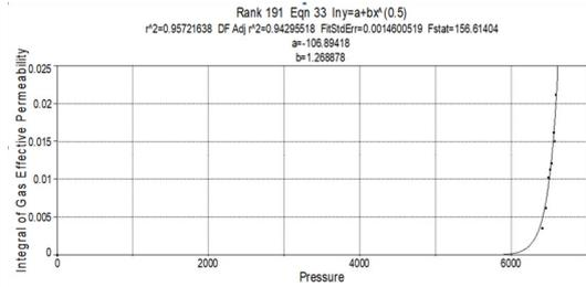
Fig. 3. Integral of gas effective permeability as a function of pressure extrapolated to zero
