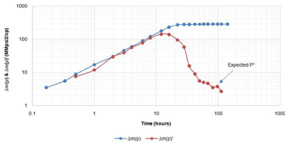
Fig. 1. Pseudopressure function and its derivative vs. time
