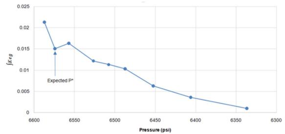
Fig. 2. Integral of gas effective permeability as a function of pressure
