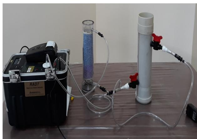
Fig. 1. Method of radon concentration measurement.
