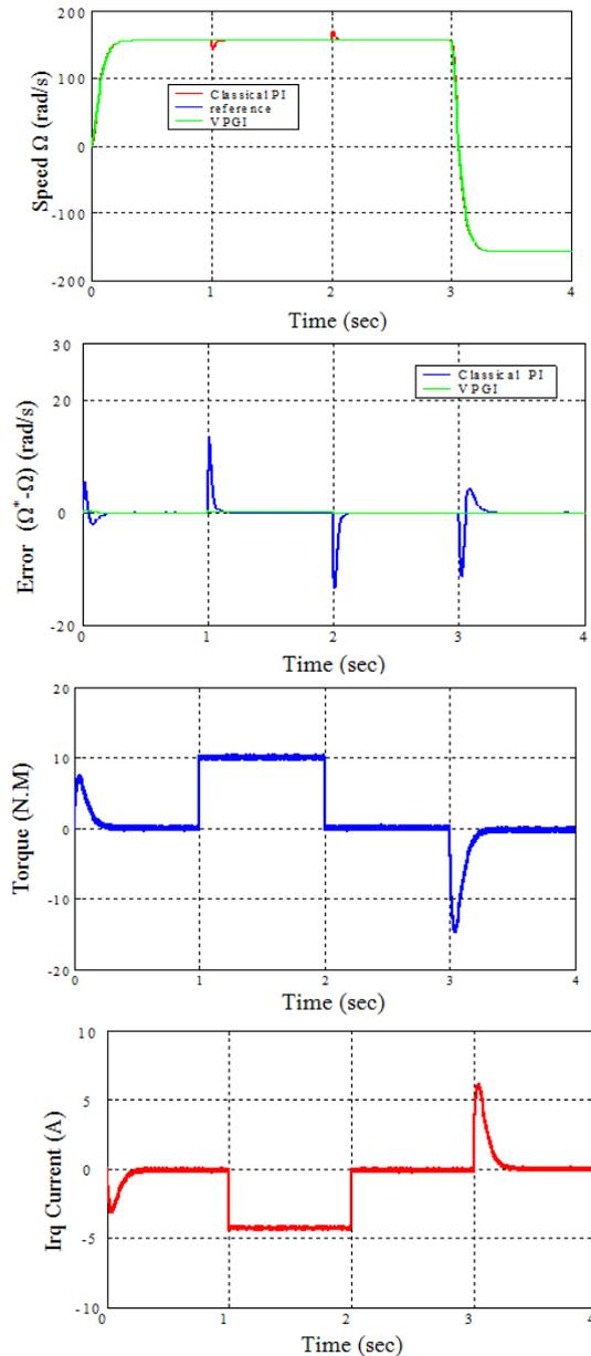
Fig. 6. Simulated results of speed control of DFIM using VGPI
