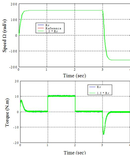
Fig. 9. Test of robustness results using VGPI for different Values of rotor resistance: nominal case and +50%.
