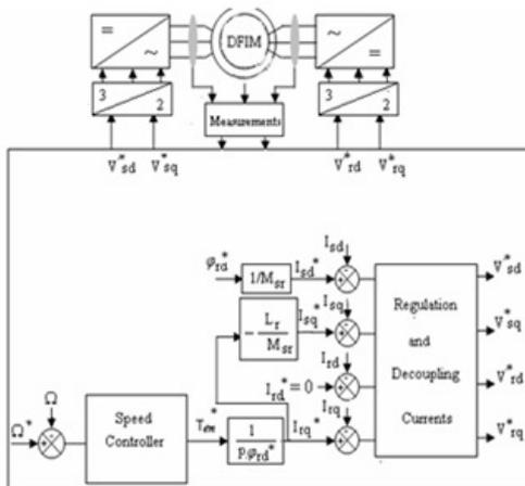
Fig. 5. Block diagram of DFIM speed control using a state space nonlinear approach.
