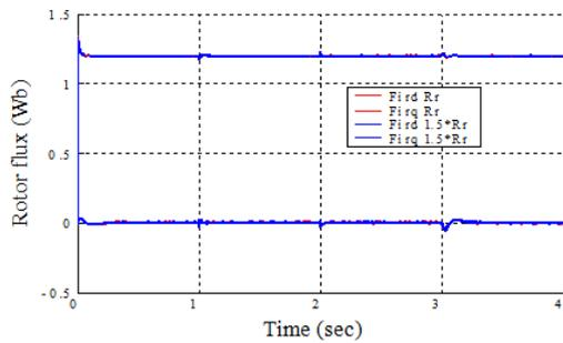
Fig. 8. Test of robustness results for rotor flux for different Values of rotor resistance: nominal case and +50%.
