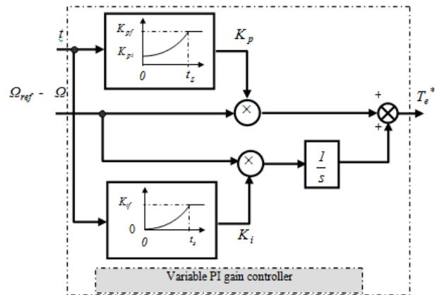
Fig. 4. The Structure of VGPI controller in DFIM vector control
