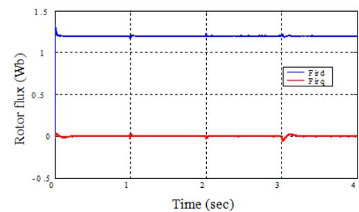
Fig. 7. Response of the two components of the rotor flux
