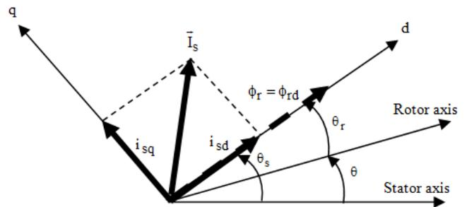
Fig. 1. Rotor flux oriented on the d axis
