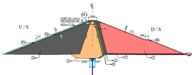
Fig. 1. Cross section of Nai Gaj dam
