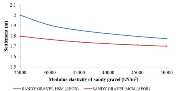
Fig. 8. Comparison of dam settlement at AFR computed with MCM (condition 1) and HSM applied to sandy gravel (condition 2)
