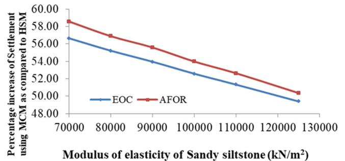
Fig. 13. Increase percentage of MCM as compared to HSM when the MOE of sandy siltstone varied from 70000 to 125000kPa
