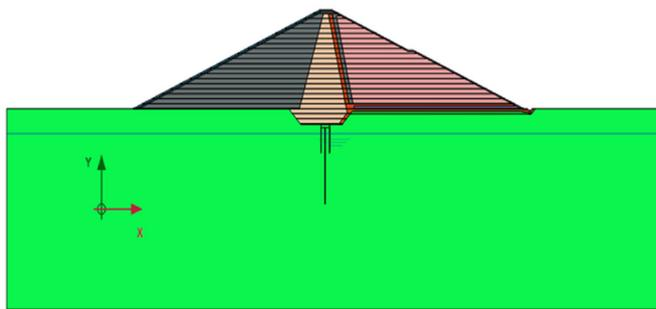
Fig. 2. Finite element model of Nai Gaj dam
