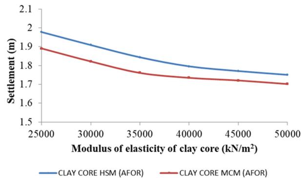
Fig. 6. Comparison of dam settlement at AFR computed with MCM (condition 1) and HSM applied to clay core only (condition 2)
