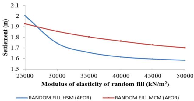
Fig. 10. Comparison of dam settlement at AFR computed with MCM (condition 1) and HSM applied to random fill (condition 2)
