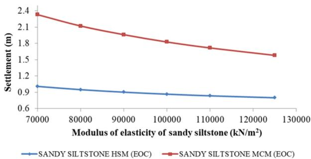
Fig. 11. Comparison of dam settlement at EC computed with MCM (condition 1) and HSM applied to sandy siltstone (condition 2)
