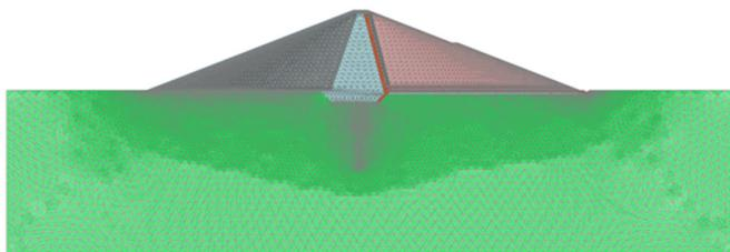
Fig. 3. Finite element mesh of Nai Gaj dam
