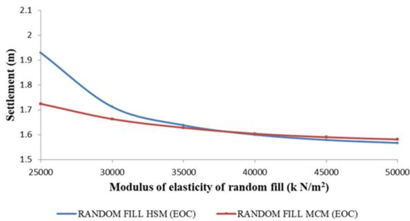
Fig. 9. Comparison of dam settlement at EC computed with MCM (condition 1) and HSM applied to random fill (condition 2)
