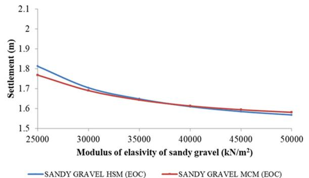
Fig. 7. Comparison of dam settlement at EC computed with MCM (condition 1) and HSM applied to sandy gravel (condition 2)
