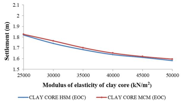
Fig. 5. Comparison of dam settlement at EC computed with MCM (condition 1) and HSM applied to clay core only (condition 2)
