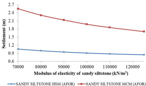
Fig. 12. Comparison of dam settlement at AFR computed with MCM (condition 1) and HSM applied to sandy siltstone (condition 2)
