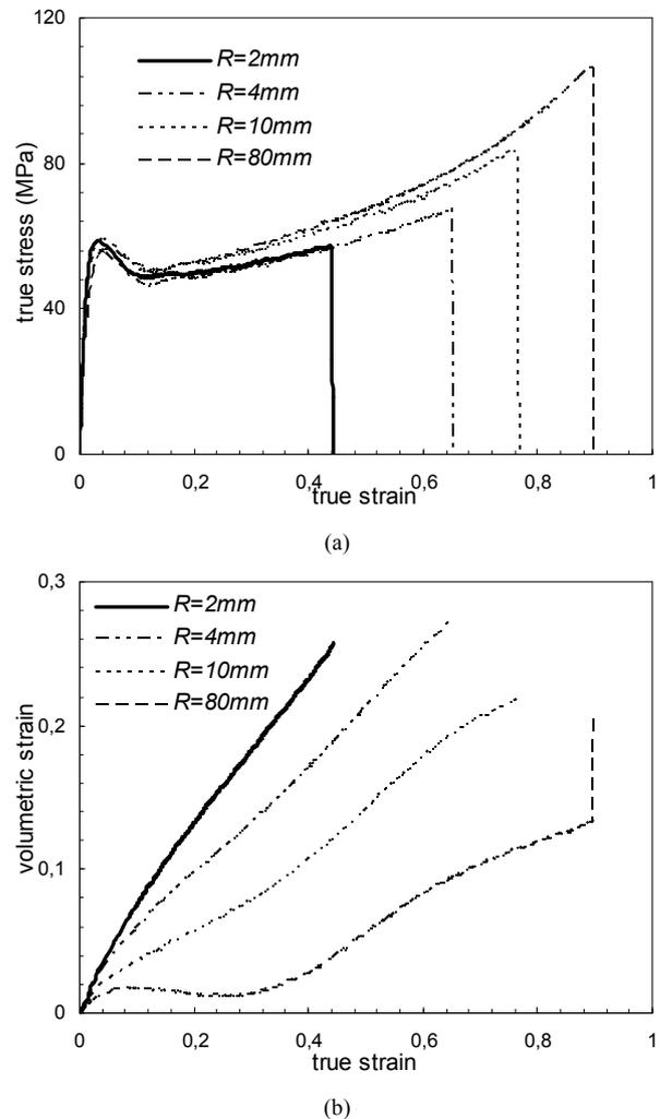
Fig. 2. Effect of stress triaxiality on (a) stress-strain response and (b) volumetric strain evolution.
