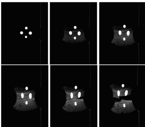
Fig. 4. Photographs of the stretching behavior under tensile testing.
