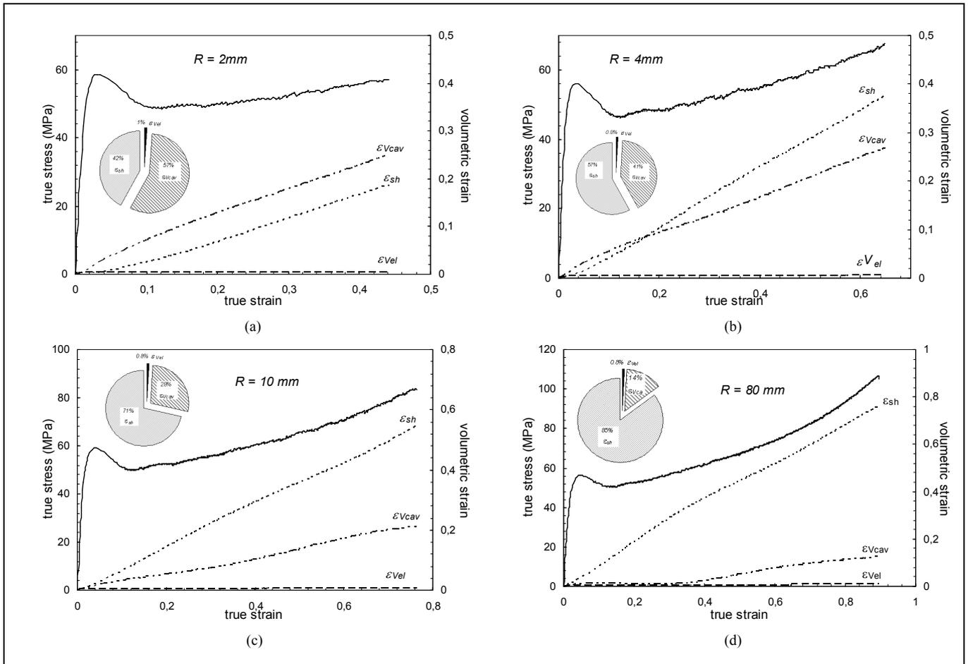
Fig. 3. True Stress and volumetric strain evolution vs true strain response.
