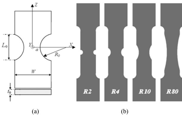
Fig. 1. Flat grooved plane stress specimen: a) the cross section b) geometry of flat specimens.
