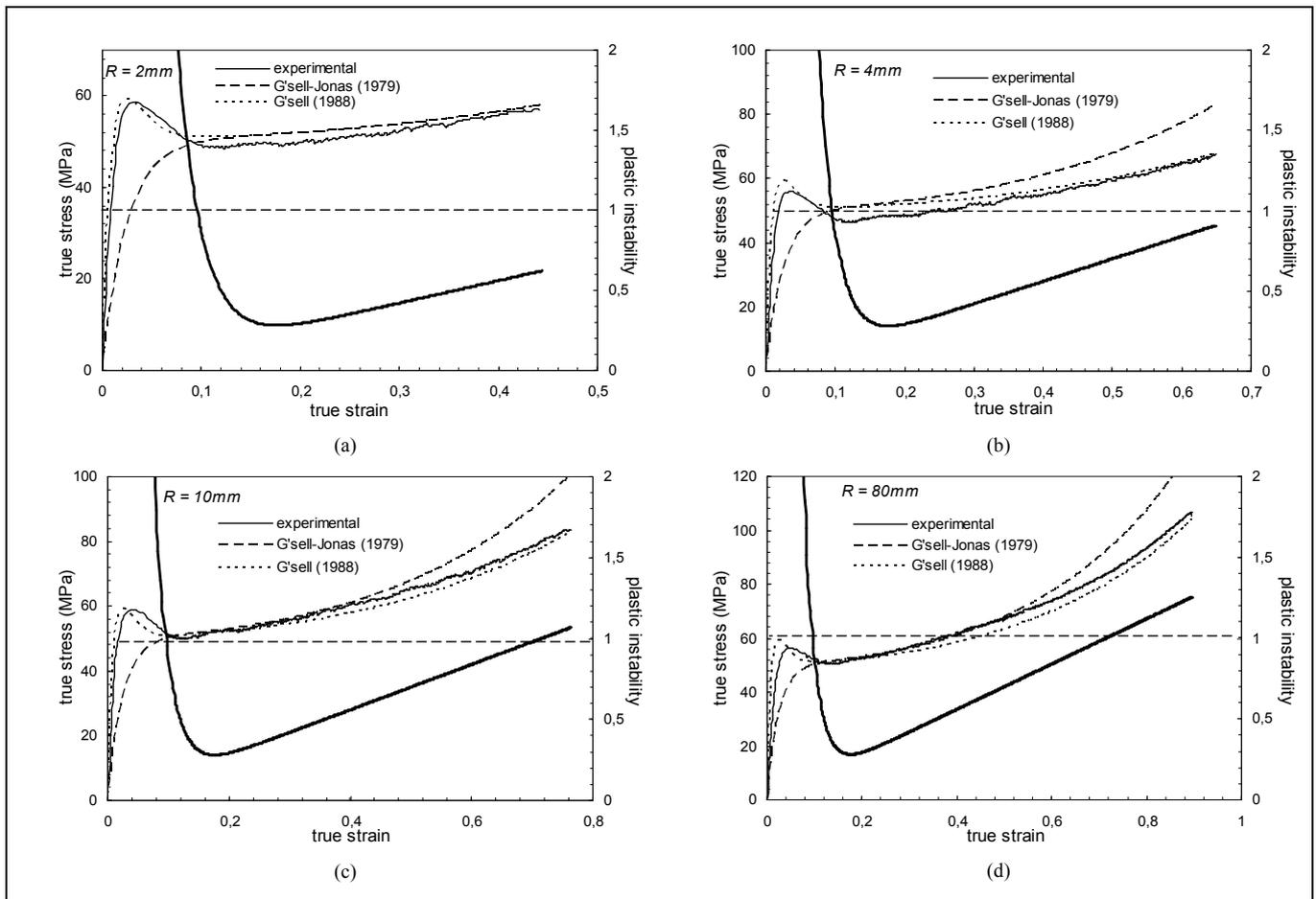
Fig. 5. True Stress and plastic instability vs true strain response.
