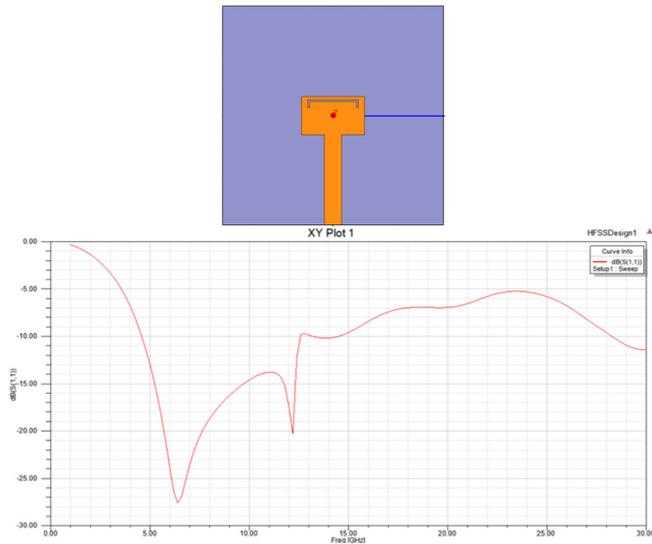
Fig. 2. Rectangular patch with U-slot. Design and results
