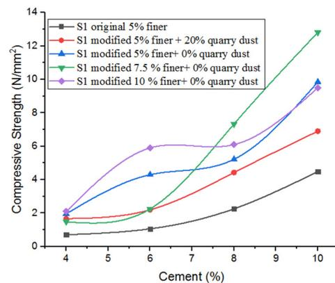
Fig. 5. 28-day compressive strength results of soil blocks with modified soil
