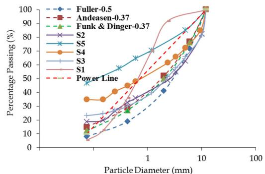
Fig. 2. Comparison of the particle distribution of the used soil with the theoretical distribution
