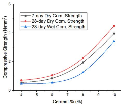
Fig. 3. Compressive strength of soil blocks with 5% fines, 20% quarry dust, and S1 Soil
