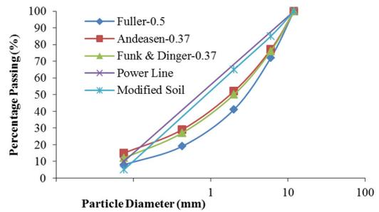
Fig. 4. Particle size distribution of the modified soil
