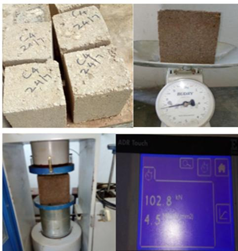
Fig. 1. Cast blocks and compressive test procedure
