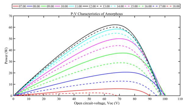
Fig. 9. Power-voltage of the amorphous module
