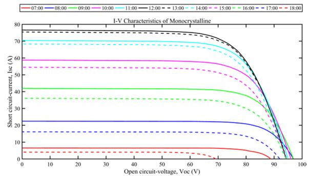
Fig. 6. Current-voltage of the monocrystalline module
