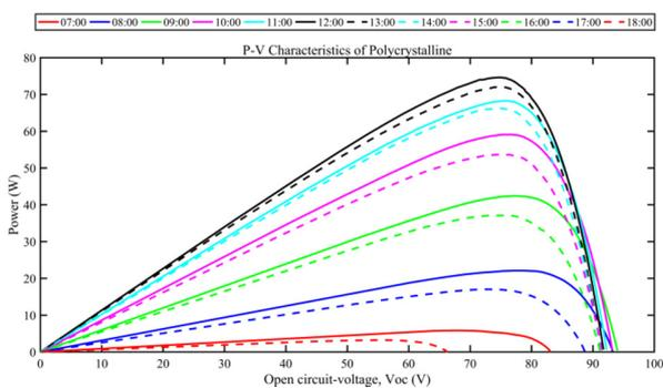
Fig. 5. Power-voltage of the polycrystalline module.
