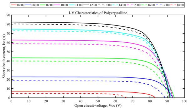
Fig. 4. Current-voltage of the polycrystalline module
