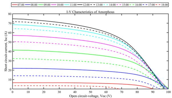
Fig. 8. Current-voltage of the amorphous module
