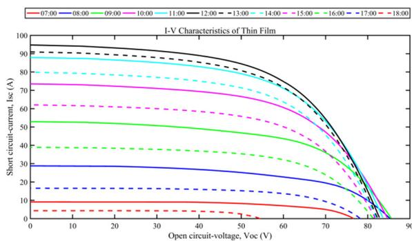
Fig. 10. Current-voltage of the thin film module
