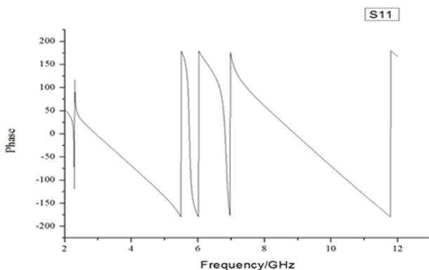
Fig. 6. Reflection phase of the proposed AMC unit cell
