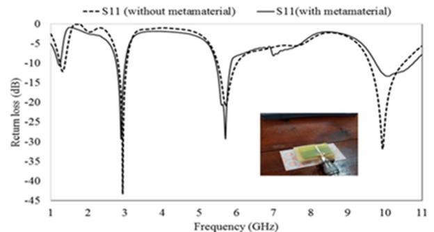
Fig. 8. Measured results of the multiband antenna with and without the AMC metasurface
