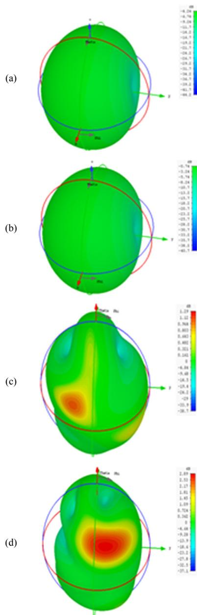
Fig. 4. Simulated gain of the proposed quad band antenna at the resonance frequencies, (a) 1.278GHz, (b) 2.8GHz, (c) 5.7GHz, (d) 10 GHz
