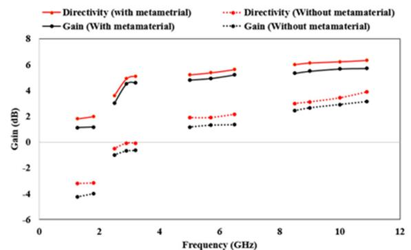
Fig. 9. Measured gain and directivity of the quad band antenna with and without AMC metasurface
