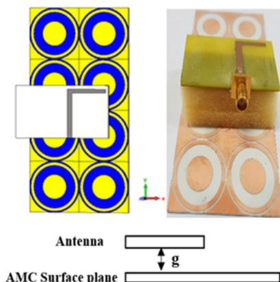
Fig. 7. Fabricated multiband antenna placed above the AMC plane
