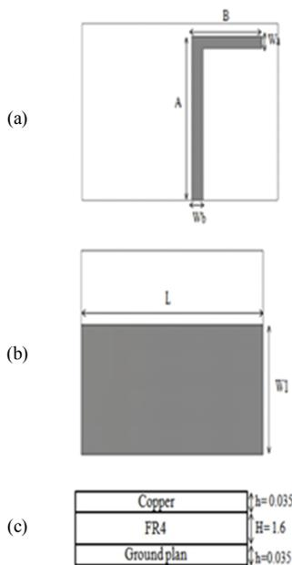
Fig. 1. The geometry of the proposed quad band antenna: (a) top view, (b) bottom view (c) left side
