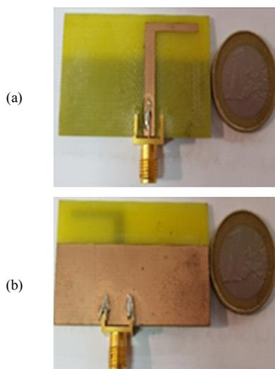
Fig. 2. The fabricated prototype of the quad band antenna, (a) Top view, (b) bottom view
