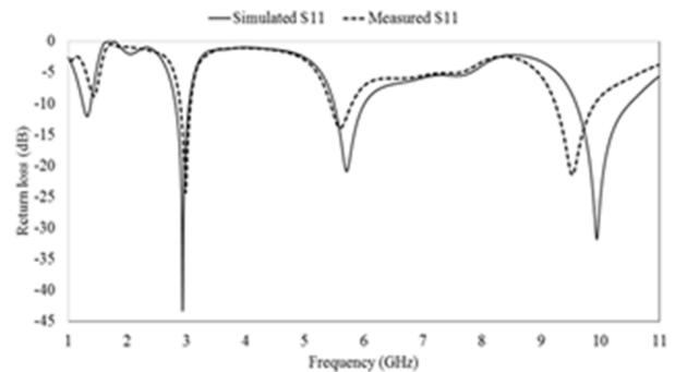
Fig. 3. Measured and simulated  $S_{11}$  result of the proposed multiband antenna without AMC
