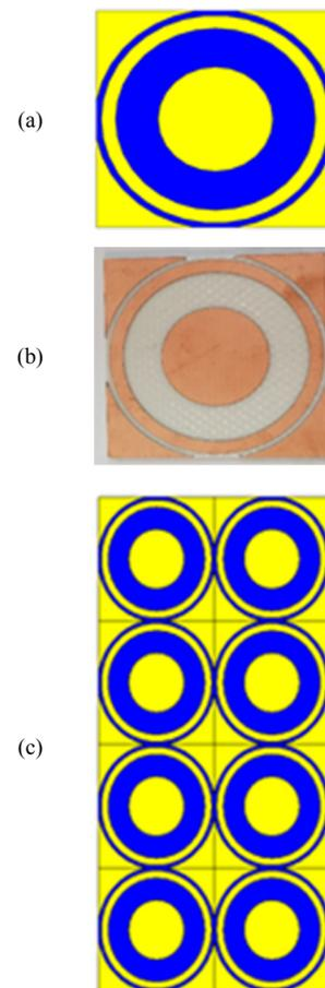
Fig. 5. The proposed AMC unit cell, (a) geometric (b) fabricated unit cell, (c) top view of the metasurface plan
