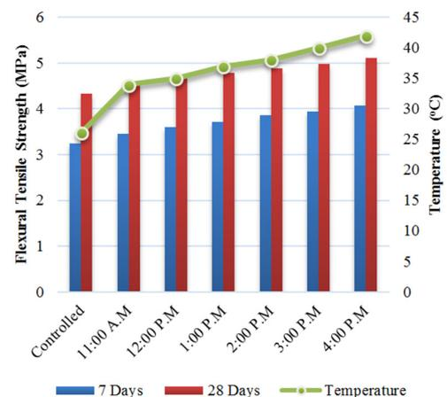
Fig. 3. Variation in flexural strength of concrete
