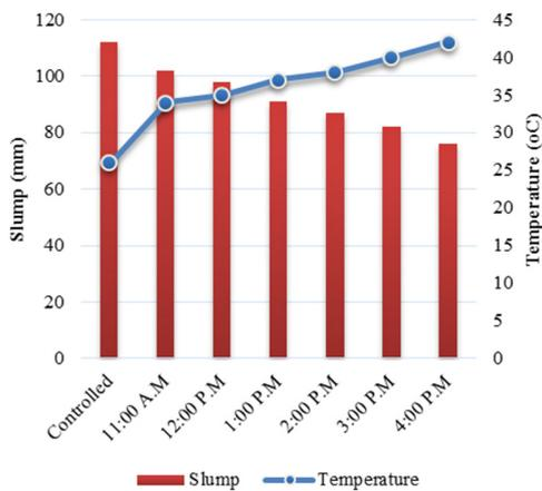
Fig. 1. Slump variation versus temperature and time
