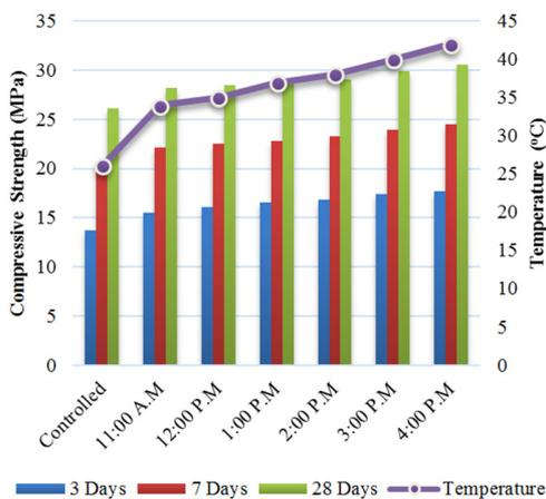
Fig. 2. Variation in compressive strength of concrete
