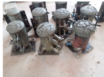
Fig. 2. Aerated concrete cylindrical specimens before trimming
