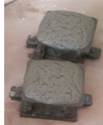
Fig. 1. Aerated concrete cubical specimens before trimming
