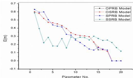
Fig. 5. Specific energy graphical representation for 6m head
