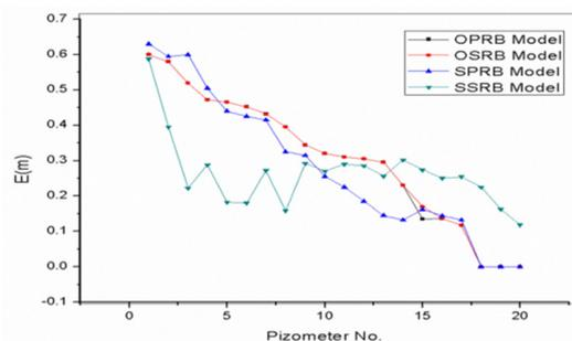
Fig. 5. Specific energy graphical representation for 6m head
