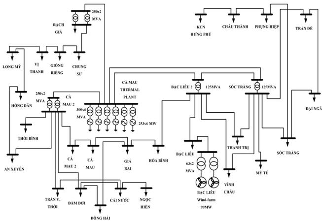
Fig. 1. Single-line diagram of the studied system.
