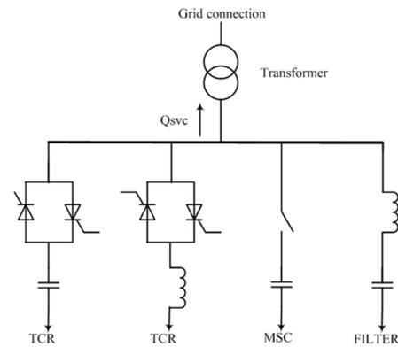
Fig. 2. Single-line diagram of SVC
