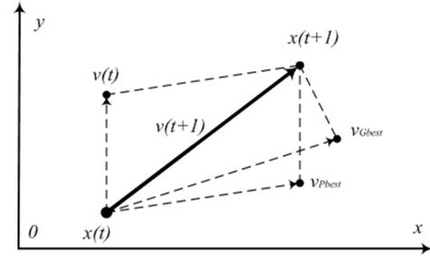
Fig. 4. Updating new position mechanism of PSO
