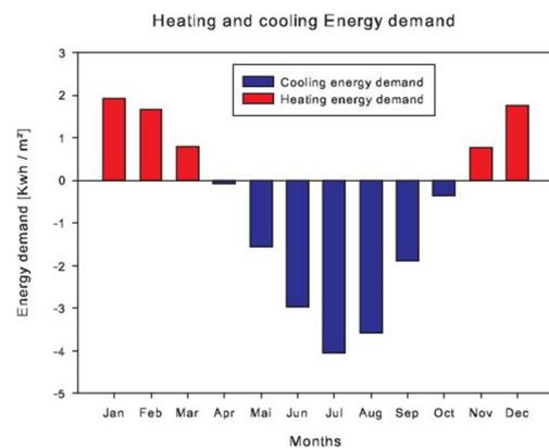
Fig. 4. Estimated heating and cooling load of the elliptic shape
