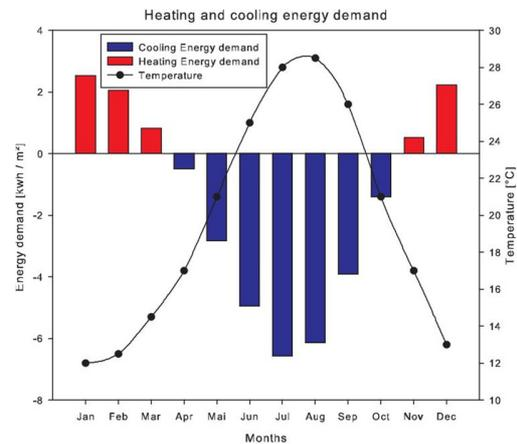
Fig. 2. Energy demand of the heating and cooling using traditional approaches
