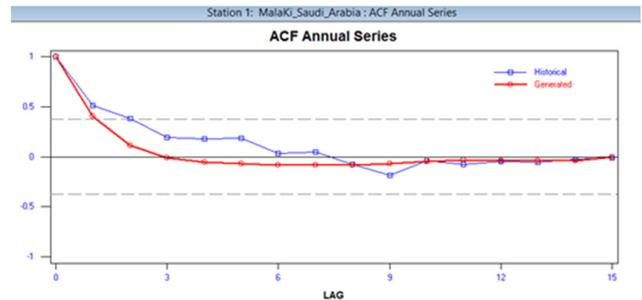
Fig. 5. Comparison between historic and generated serial correlation for an ARMA(2,1) model.
