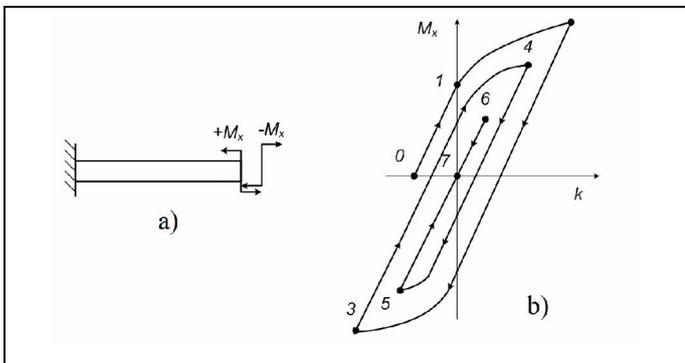
Fig. 2. a) Loading condition and b) deformation diagram of a wire in the course of straightening
