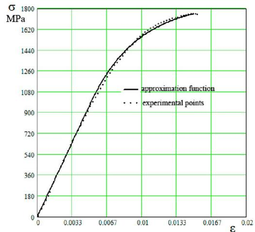
Fig. 3. Experimental stress-strain diagram and approximation function
