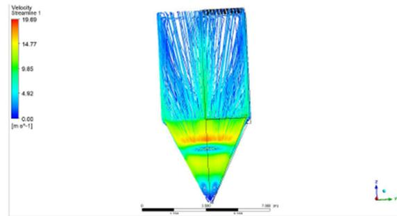
Fig. 6 Current lines on the opposite side of the hopper inlet
