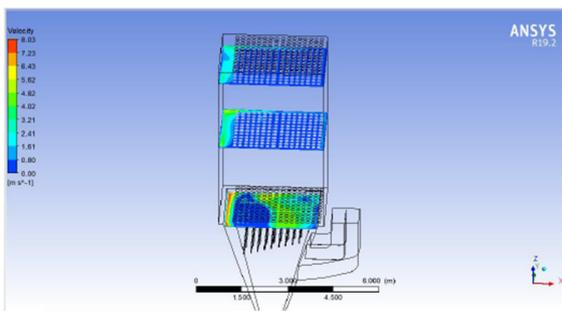
Fig. 9 Velocity profile for the proposed alternative geometry
