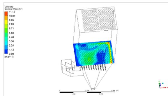
Fig. 7 Profile of velocities in the plane just before the baghouses
