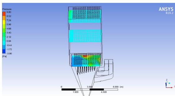
Fig. 10 Pressure profile for the presented alternative
