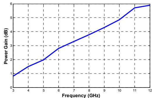
Fig. 5. Simulated power gain of the proposed antenna
