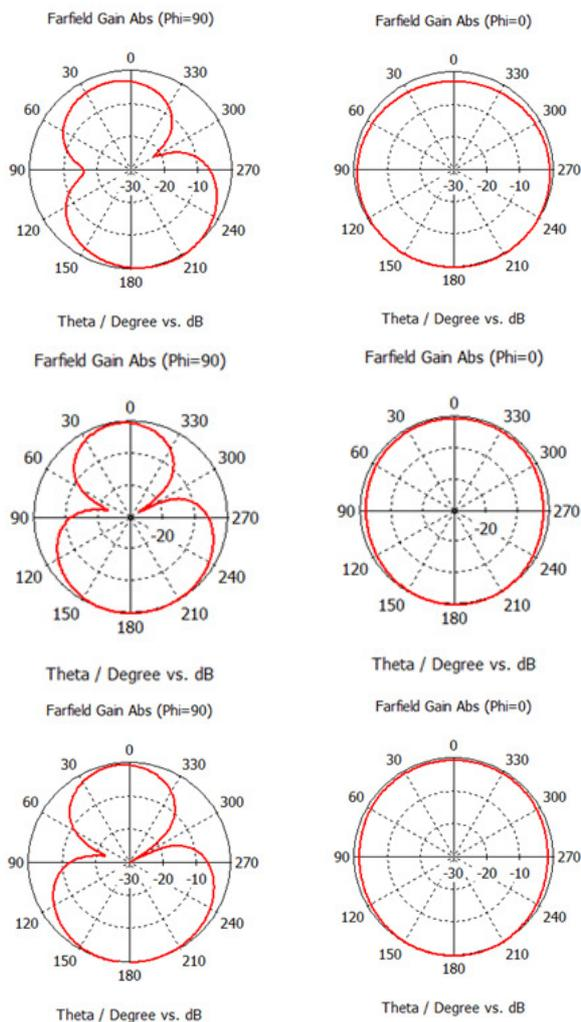
Fig. 6. Normalized radiation pattern for E and H planes in polar form at the resonant frequencies
