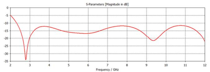
Fig. 3. Simulated reflection coefficient S11 vs operating frequency
