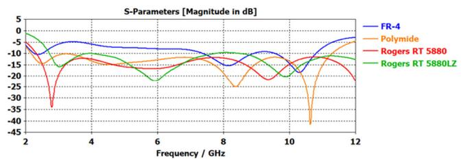
Fig. 4. Reflection coefficient S11 vs operating frequency for several substrate materials: Rogers RT 5880 ( $\epsilon_r=2.2$ ), Rogers RT 5880Lz ( $\epsilon_r=1.9$ ), FR-4 ( $\epsilon_r=4.3$ ), and Polyimide (3.5)
