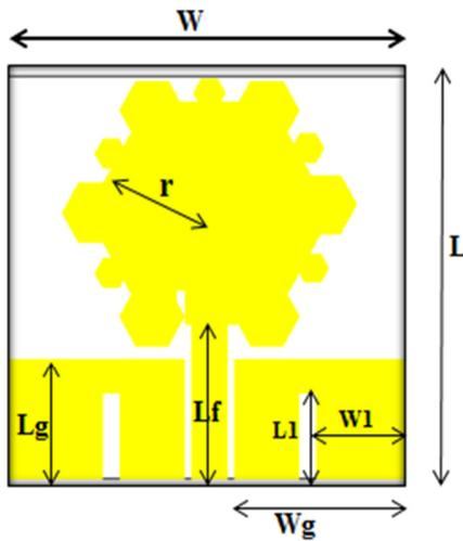
Fig. 1. Design of monopole antenna configuration with labeled parameters
