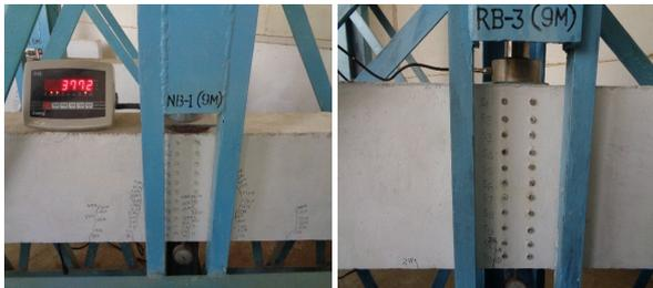
Fig. 1. Beams mounted on loading frame.
