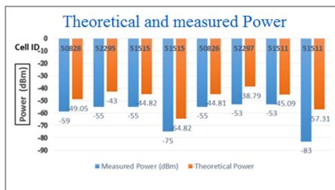
Fig. 8. Measured and theoretical power for tested cell
