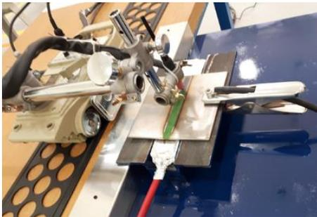
Fig. 1. Experimental setup of TIG welding with flux paste (a motorized carriage, torch-workpiece).
