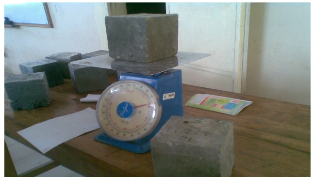
Fig. 3. Weighing process to determine densities of concrete samples
