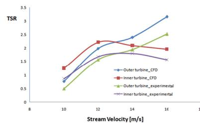
Fig. 16. Tip speed ratio variation within stream velocity
