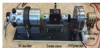
Fig. 6. PMG testing bench
