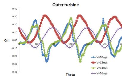
Fig. 14. Momentum coefficient variation for the outer turbine
