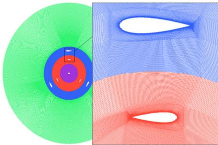
Fig. 2. Mesh of the CR-VAWT concept
