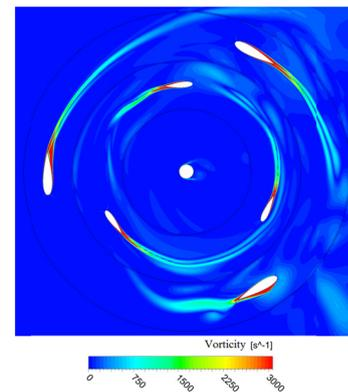
Fig. 13. Vorticity magnitude for theta 90 degrees, for V=12m/s
