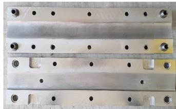
Fig. 3. Blades molds for inner turbine
