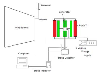
Fig. 8. Schematic diagram of experimental system
