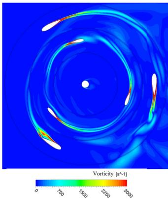
Fig. 11. Vorticity magnitude for theta 30 degrees, for V=12m/s
