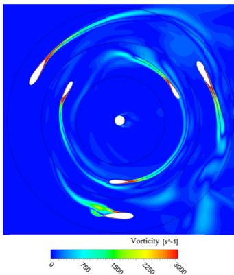
Fig. 12. Vorticity magnitude for theta 60 degrees, for V=12m/s
