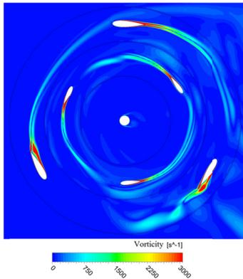
Fig. 10. Vorticity magnitude for theta 0 degrees, for V=12m/s
