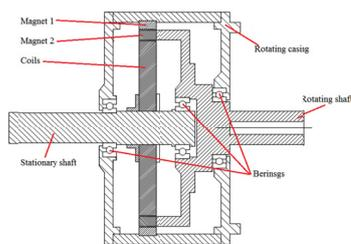
Fig. 4. PMG cross section
