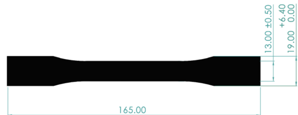
Fig. 1. Tensile sample shape and dimensions in SolidWorks 2023.
