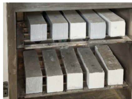
Fig. 2. Accelerated carbonation chamber.
