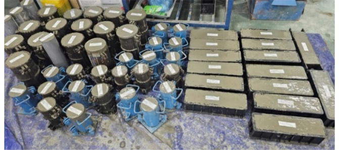
Fig. 1. Fabrication of specimens for carbonation resistance determination.
