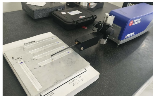
Fig. 2. Surface roughness measurement procedure.
