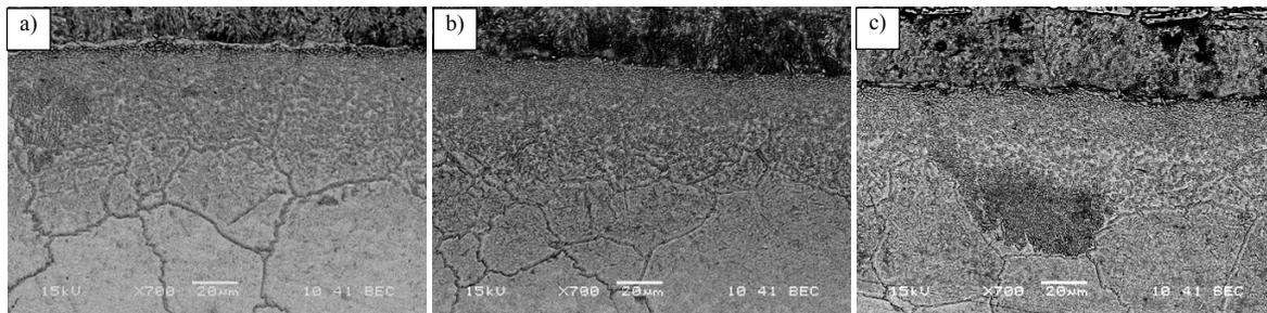
Fig. 7. Stainless steel region of bimetal casting for a) as-cast; b) 60min annealing time and 760°C annealing temperature and c) 180min annealing time and 760°C annealing temperature.
