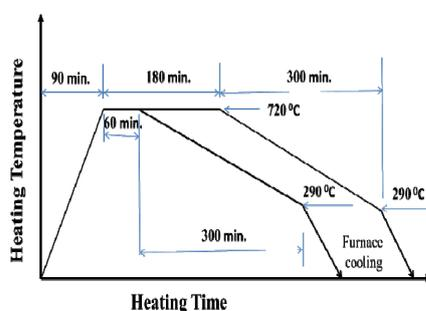
Fig. 1. Schematic illustration showing low temperature annealing heat treatment processes applied for bimetal castings.
