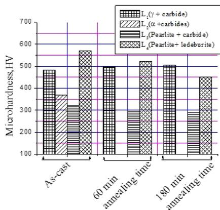
Fig. 8. Hardness measurements of interface layers of as-cast, annealed for 60min and annealed for 180min bimetal casting.
