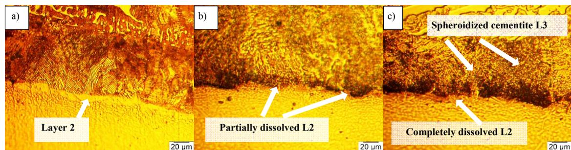
Fig. 4. Differences in annealed interface microstructures: a) as-cast, b) 60min annealing time, c) 180min annealing time.
