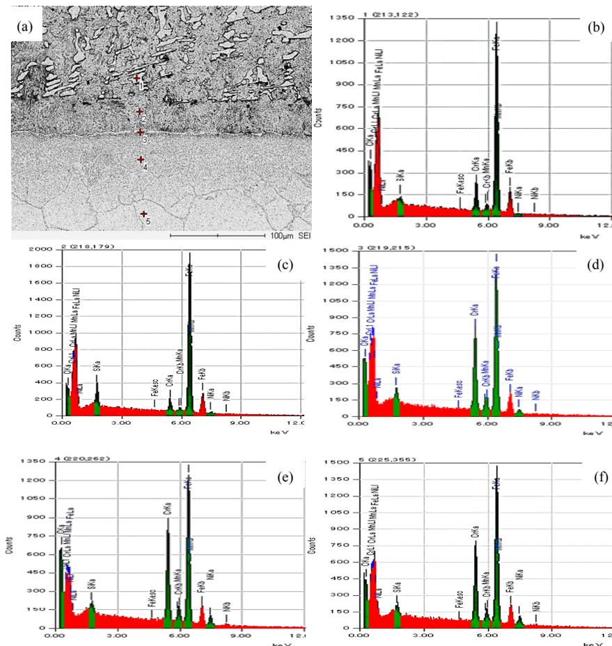
Fig. 5. EDS analysis for interface layers of as-cast ductile cast iron/stainless steel bimetal casting, a) as-cast interface microstructure, b), c), d), e) and f) are the point 1, 2, 3, 4 and 5 EDS analyses respectively.
