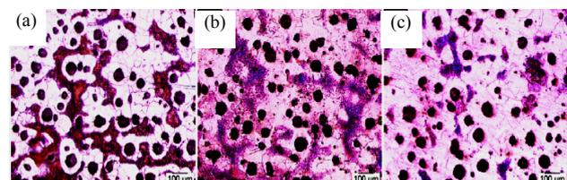
Fig. 2. Microstructure of ductile iron region of bimetal casting for a) as-cast, b) 60min annealing time, c) 180min annealing time.
