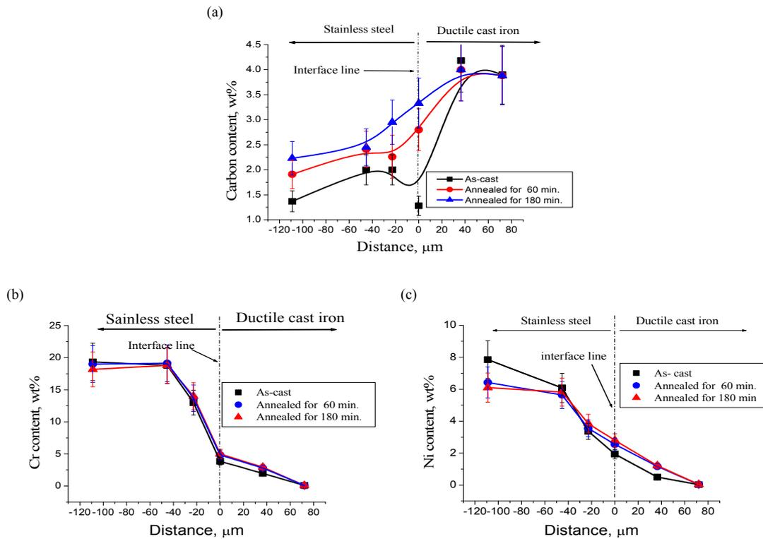
Fig. 6. Interface C, Cr and Ni distribution for as-cast and annealed ductile cast iron/stainless steel bimetal casting; a) C%; b) Cr% c) Ni%.
