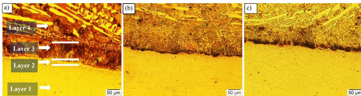
Fig. 3. Microstructure of interface region of bimetal casting for a) as-cast, b) 60min annealing time, c) 180min annealing time.
